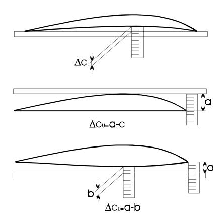
Fig. 2 Distortions of hydrofoil profiles
