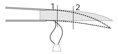
Fig. 5 Thermal bending of a trailing edge
