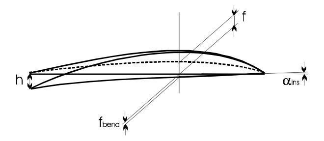
Fig. 4 Influence of bending on the attack angle
