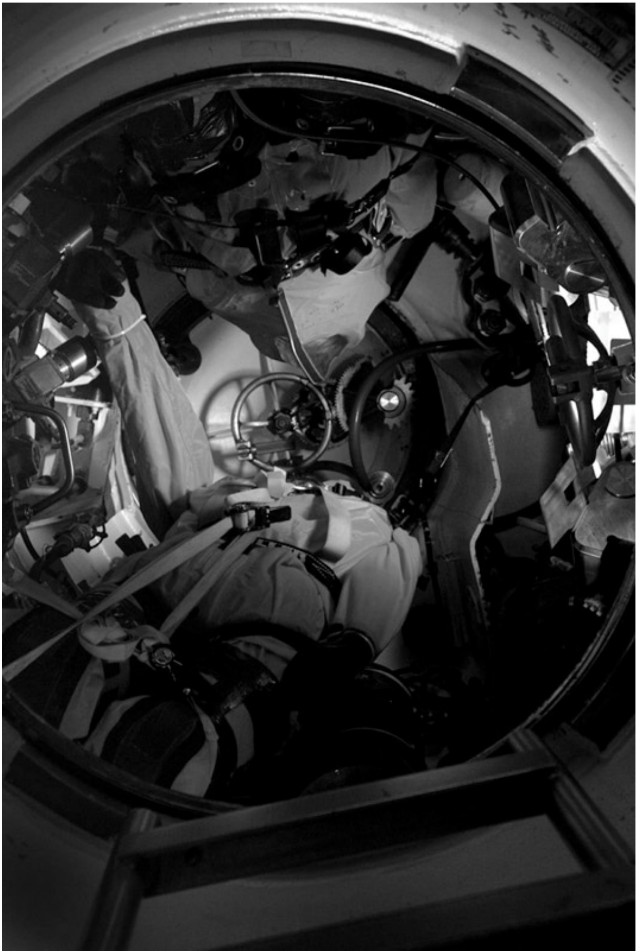
Instrument mannequins dressed in Submarine Escape Immersion Equipment (SEIE) seen inside the engine-room escape trunk of the US Navy submarine Virginia (SSN-774) in August 2004 during a series of pre-commissioning trials. SEIE is designed to allow safe escape from a submarine up to depths of around 200m. Survivors on a
