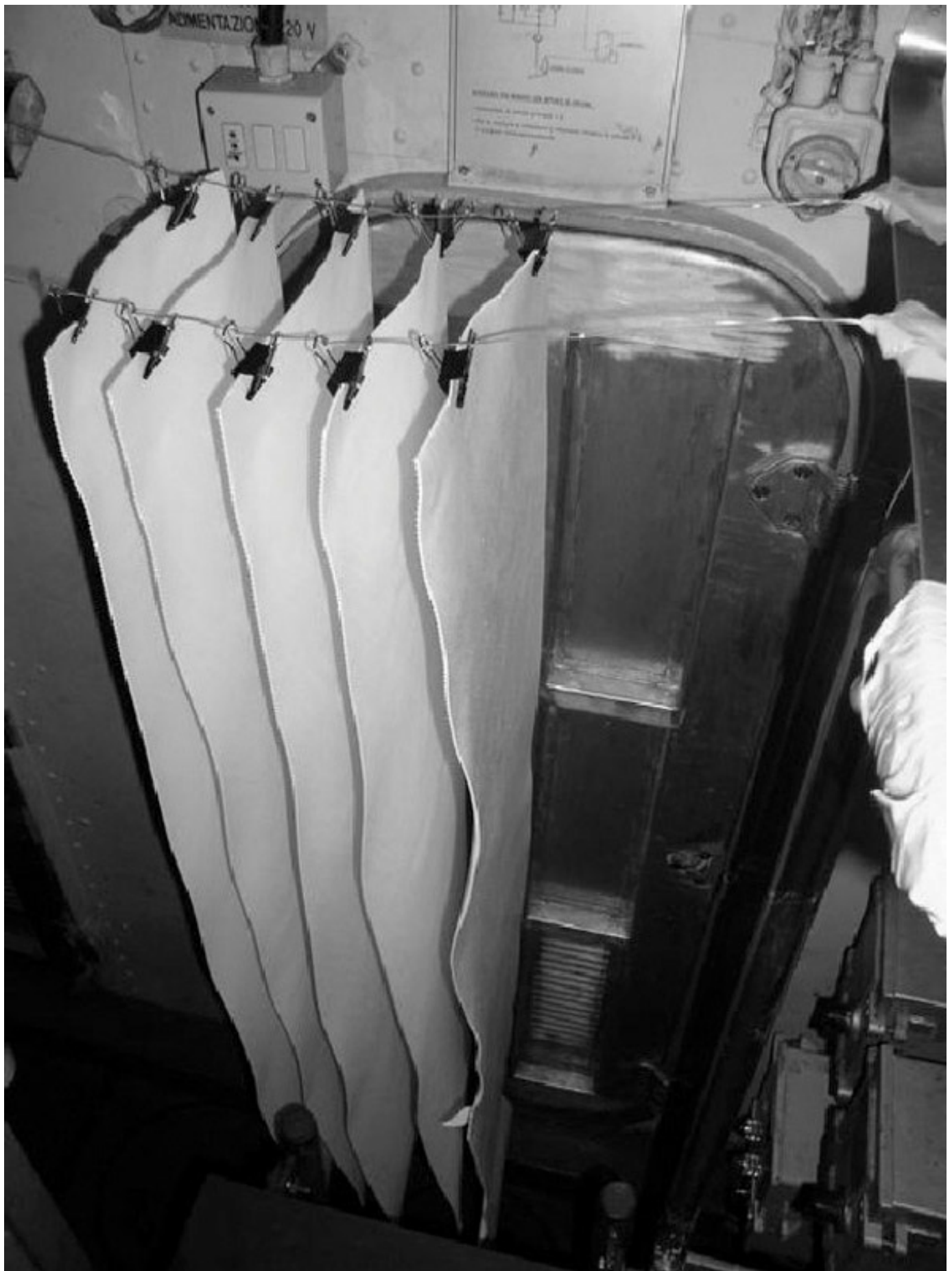
Artificial means – such as the use of carbon monoxide absorbent materials like these ExtendAir lithium hydroxide curtains manufactured by America's Micropore – can be used to help control carbon monoxide buildup on a distressed submarine. ( Micropore Inc. )
