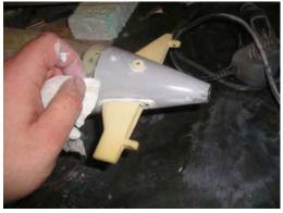
• Fill small scratches or pin holes found in the hull finish or from the last step of filling with the air-dry putty. Again, use only enough to fill the blemish. Too much
