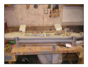
Note: You can always drill more holes in these formers to allow for water and air flow passage later for better performance. When doing so, be sure not too drill too big or too close to the inside edge, thereby weakening the bulkhead
