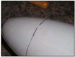
• Mask off all the surfaces that are not to be glued on the lips. It might be a good idea to mask of the outside of the hull as well
