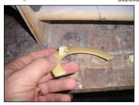
Cut the hull formers at the designated cut lines (It's possible this might already be done). The bottom formers are designated by the little wart located on the side
