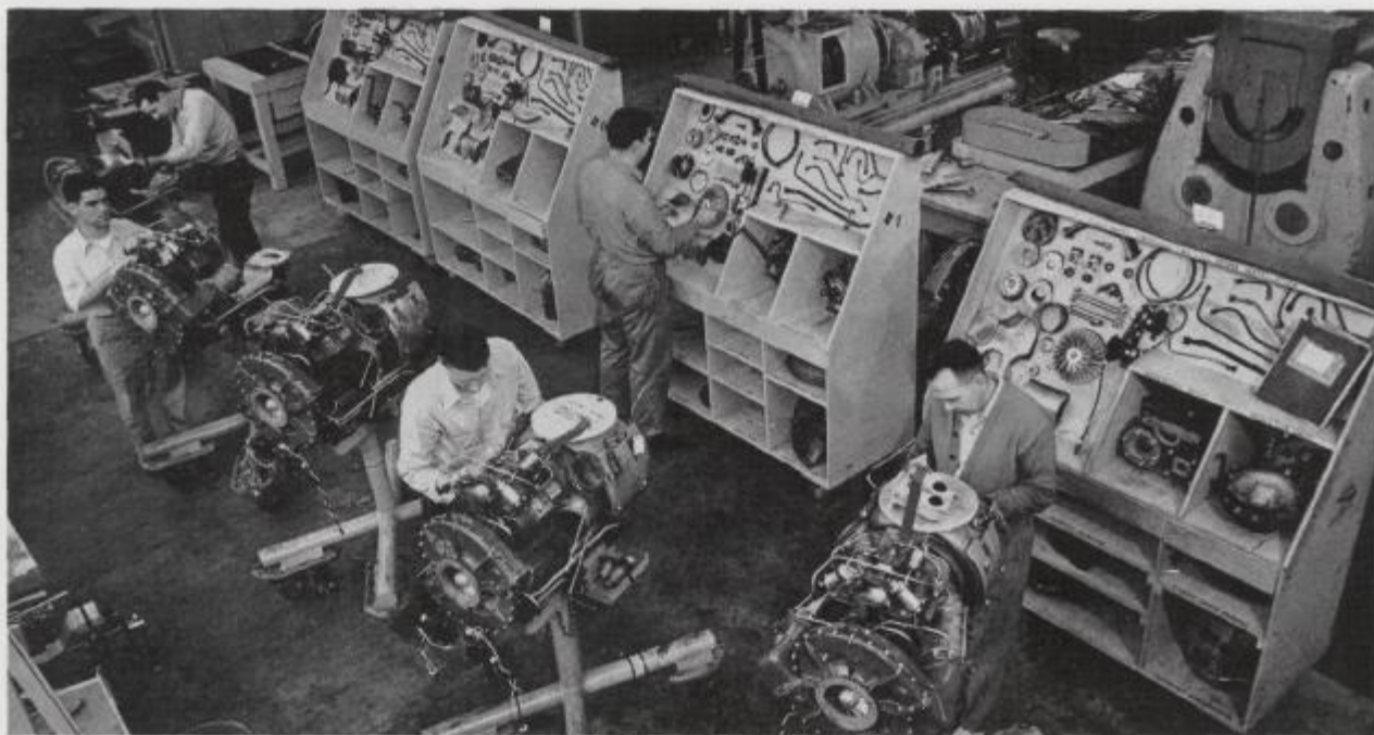
Gas turbine engines were produced on a limited assembly-line basis during the year. Substantial progress was made in cutting production cost and increasing engine efficiency.
