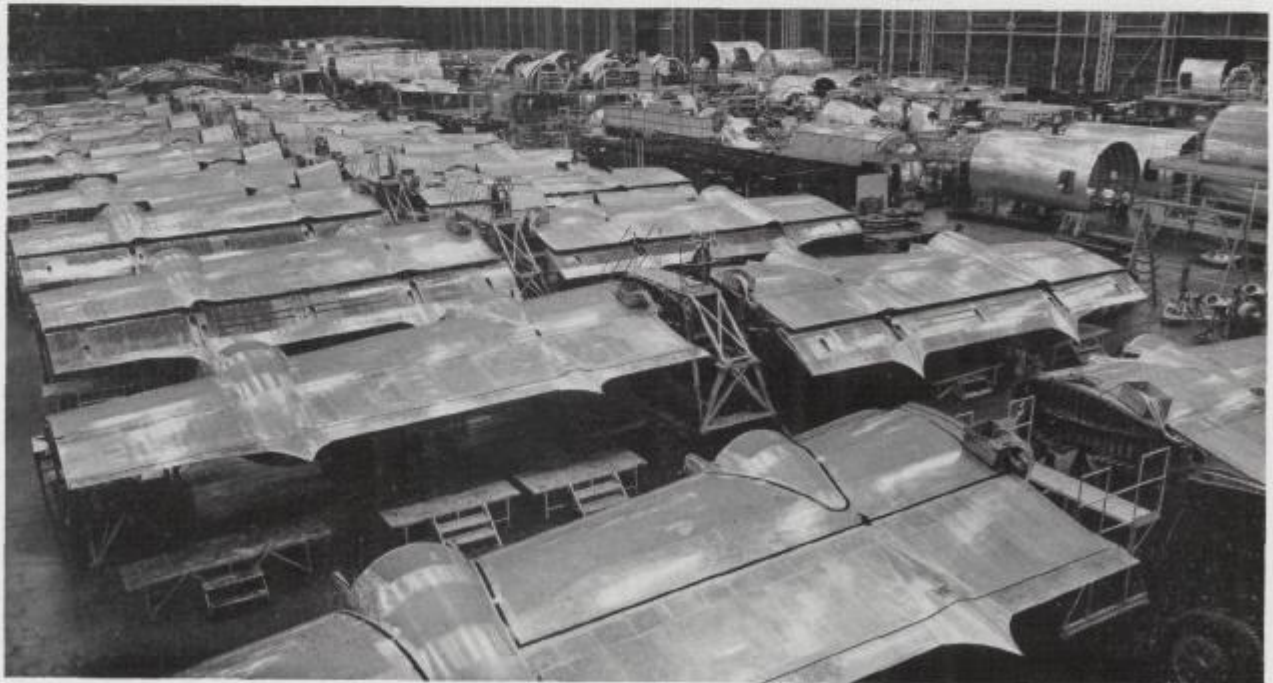
Inboard wing sections of the KC-97 Stratofreighters move along the assembly lines at Boeing plant at Renton, Washington. Production was gradually increased during the year.
