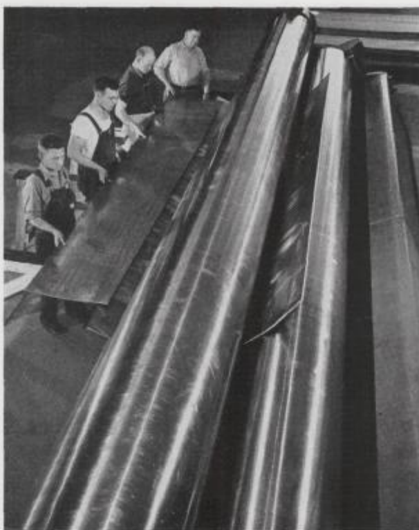
High-performance jet aircraft require manufacturing techniques previously unknown to aircraft industry. This huge pincher-type bending roll is used to contour B-47 wing skin.
