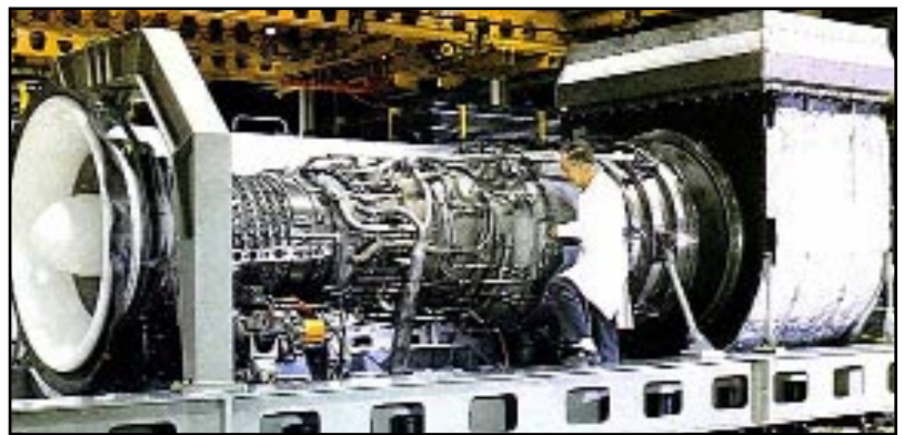
LM-2500 GAS TURBINE (33,600 HP)
