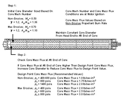
A major advantage of using combined core Mach number/core mass flux erosive burning design criteria for either non-erosive or max recommended erosivity motor designs is that irregardless of whether the motor propellant is sensitive to velocity-based or mass flux-based erosive burning, provisions for both have been included as both core Mach number limits and core mass flux limits have been considered.
