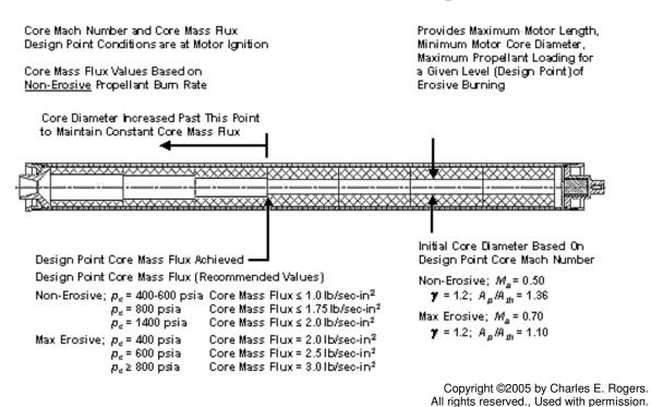
As shown in the figure above, when using the constant core mass flux core design, once a design point core mass flux is achieved, the core is then opened up (the core
