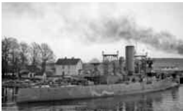
Two images of Harald Haarfagre during her conversion into Thetis at Kaldnes Mekaniske Verksted at Tønsberg. Structural work is complete but she still lacks her armament, directors and searchlights, which will be installed at Kiel. (Dirk Nottelmann collection)
