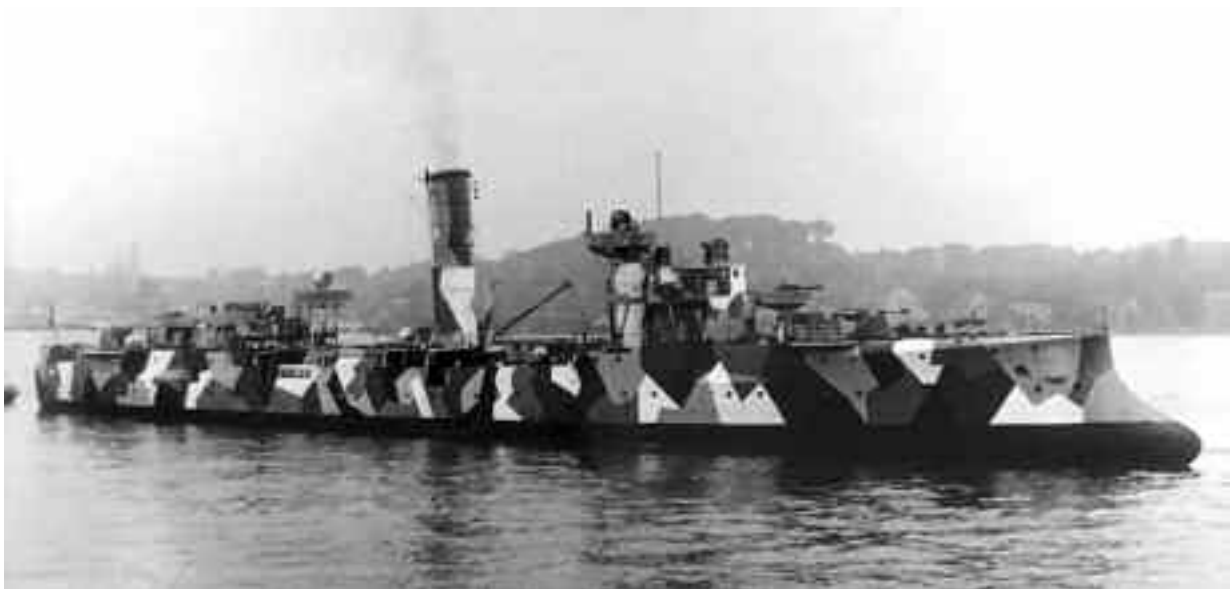
Arcona in the spring of 1940, fresh from her reconstruction. She is wearing the first of her many different camouflage schemes (see below). Note the guardrail-lined sponsons for the 10.5cm guns, which would soon be closed by bulwarks. (Dirk Nottelmann collection)
