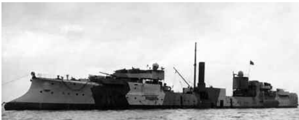
Medusa during the second half of 1941 after her first minor conversion, which included the mounting of splinter shields on the 3.7cm guns and the partial enclosure of the searchlight platforms. (Dirk Nottelmann collection)
