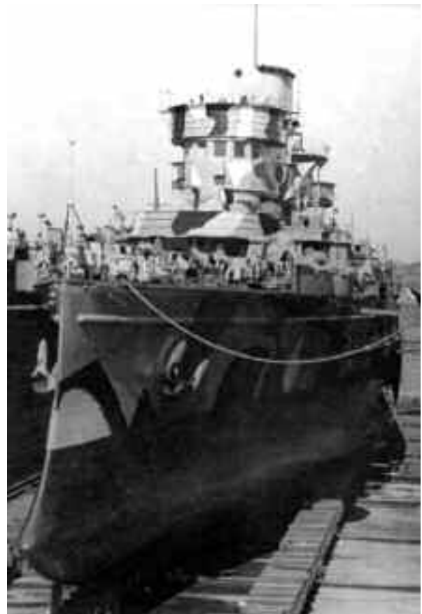
Nymphe in dry dock at Kiel, with her initial(?) camouflage pattern. Her degaussing coil is prominent; this was carried farther down the side of the hull than the deck-edge installation of Thetis . (Dirk Nottelmann collection)
