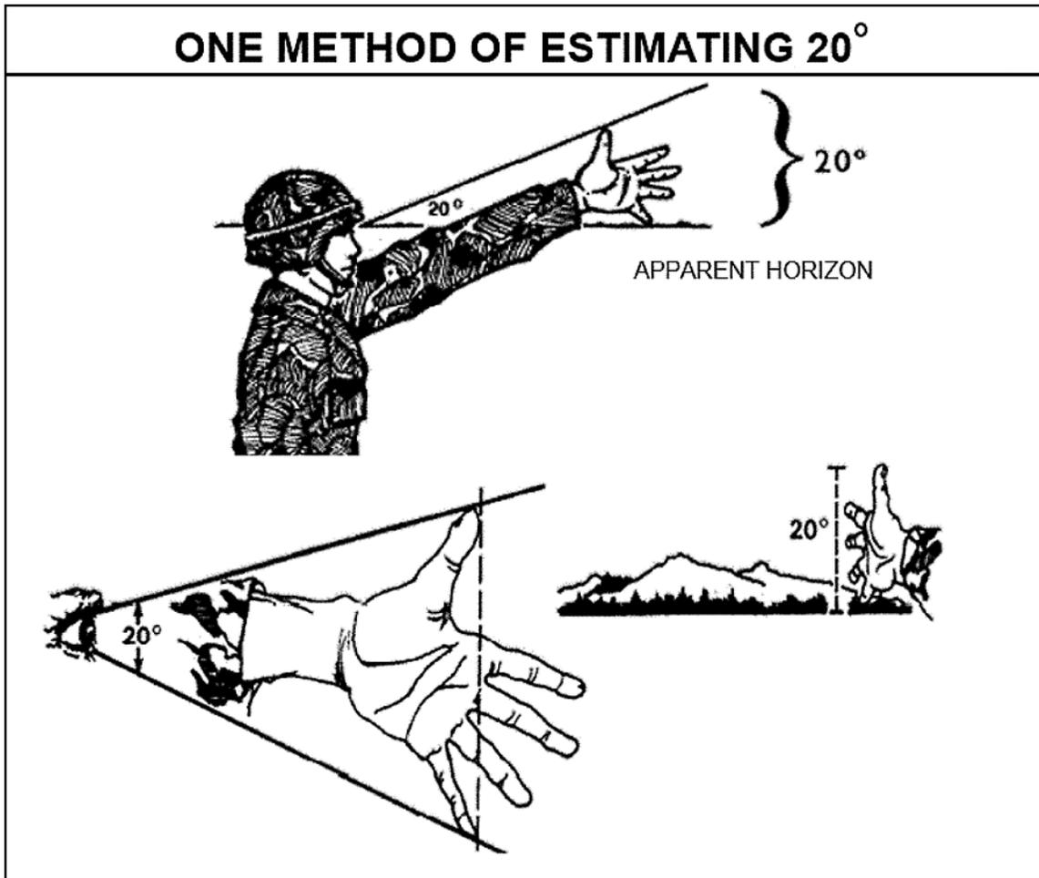
**Figure 3-1. A method of estimating 20 degrees**
