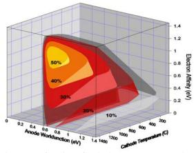
**Figure 3**: Theoretical PETE efficiency as a function of cathode temperature, anode work function, and cathode electron affinity.  $E_g$  is fixed at 1.4 eV, the number of collisions with the surface is  $10^4$ , and the anode temperature is  $327^{\circ}$ C.
