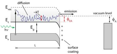
Figure 1: Schematic of the PETE process. Thermal energy assists photoelectron emission, harvesting both photon and thermal energy in the process
