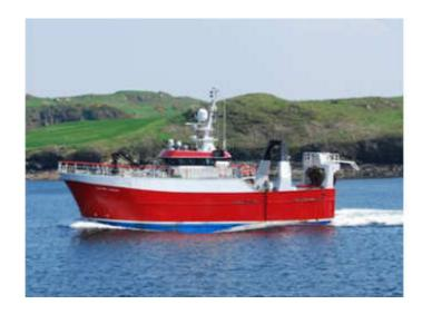
Type: Wet fish trawler, twin rigged, with stern ramp
