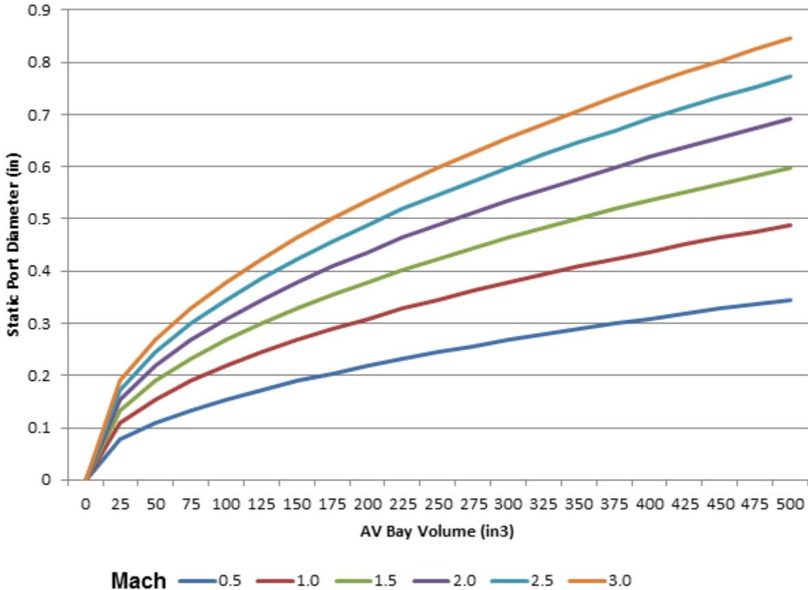
**Figure 7 – Single Port Size by Mach Velocity**
