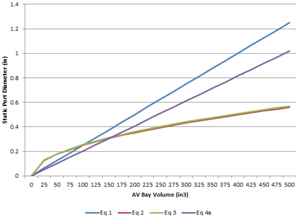
Figure 2 – Single Static Port Sizing
