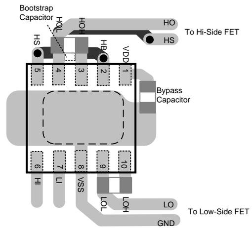
Figure 25. WSON-10 With HOH and LOH Gate Resistors
