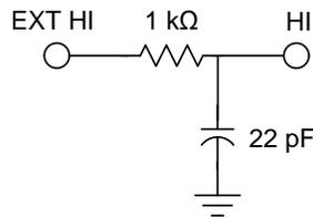
**Figure 16. Input Filter 1 (High-Side Input Filter)**
