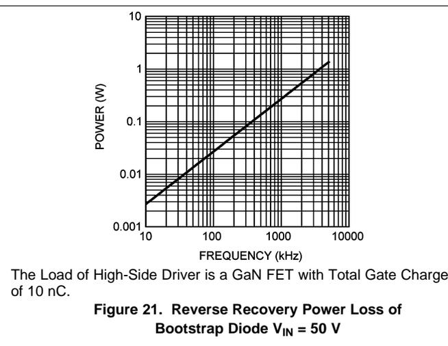
Figure 21. Reverse Recovery Power Loss of Bootstrap Diode  $V_{IN} = 50 V$
