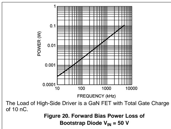
Figure 20. Forward Bias Power Loss of Bootstrap Diode  $V_{IN} = 50 V$
