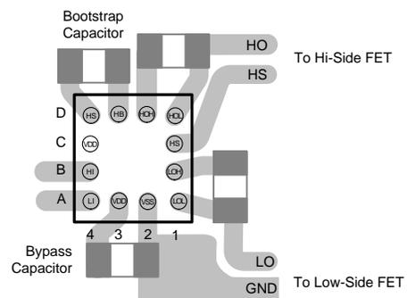
Figure 27. DSBGA With HOH and LOH Gate Resistors
